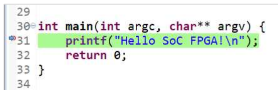
Figure 6-44. Stop at breakpoint
